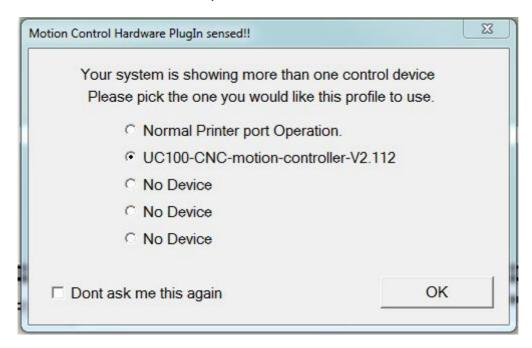
Select the UC100 CNC motion controller from the list.
