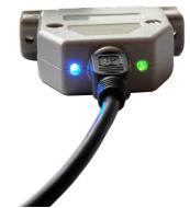
The 2 LEDs on the backshell of the UC100 controller.
